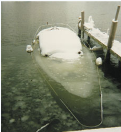
A plastic thru-hull that was an inch or two above the waterline cracked and the weight of the snow lowered the damaged fitting to just below the surface. The boat gradually filled with water and sank.
