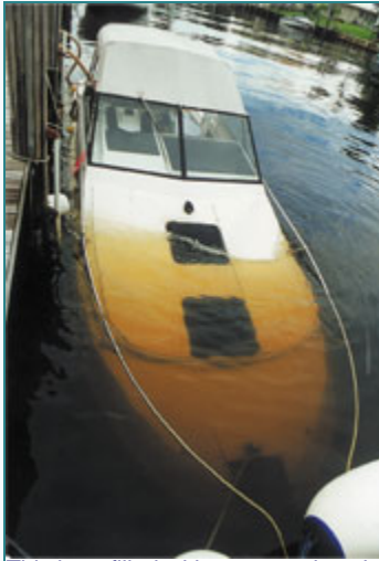
This boat filled with water and sank because the scuppers were clogged with leaves.
