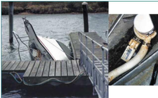
It doesn't take much to hold a float switch down. Switches should be oriented so that they are clear from interference and secured to the bilge floor. This boat sank when its bilge pump switch was blocked by the hose.
